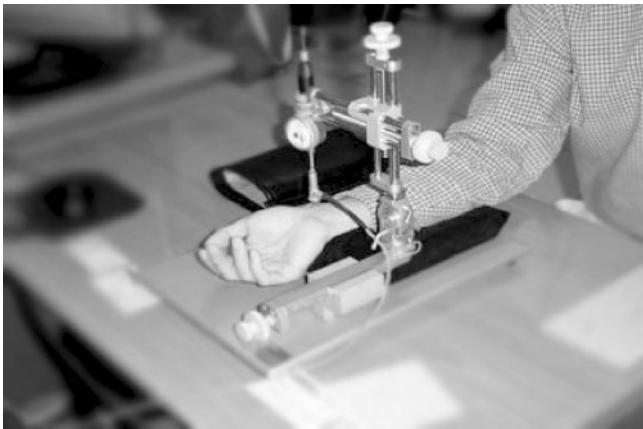
Figure 1. The acquiring instrument of blood pressure waveform.
